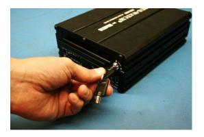
2) Connect the Hard Drive to the computer using the provided USB Cable.
